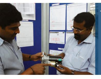
Starter Motor with Thermal Protection: Starter motor with autocut off & auto-reset feature - protection against thermal overload.
