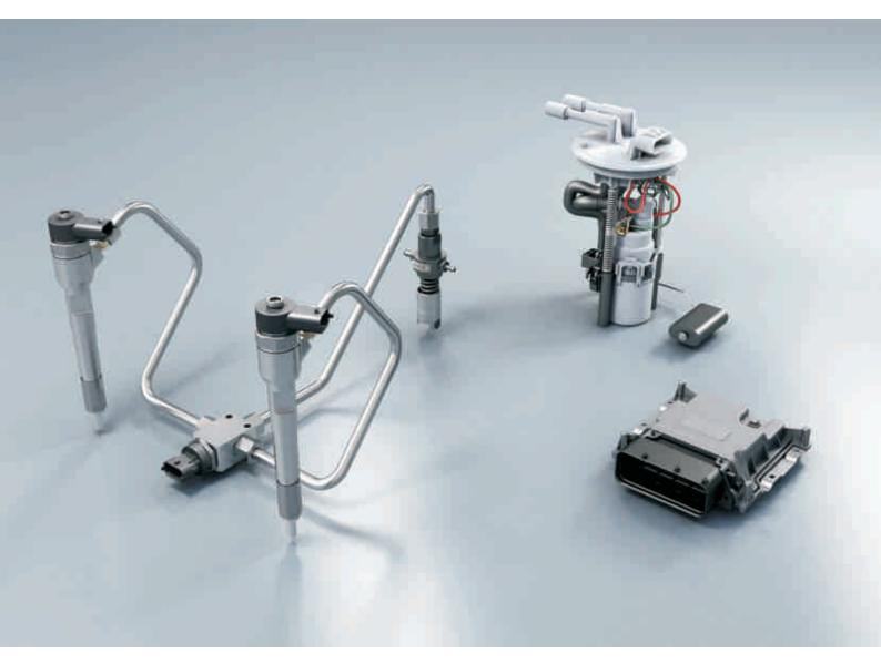
Third Generation CRS1-14 Unit Pump, with solenoid injector, fuel distributor block and feed pump control capable of 1450bar pressure, having locally developed Engine Control Unit embedded with customized software functions.
